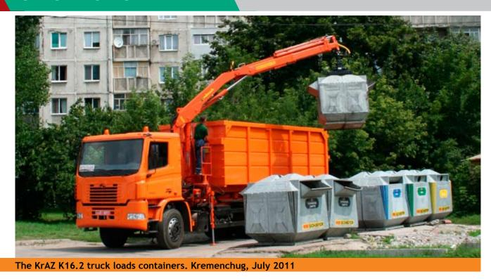
First domestic prototypes such as KrAZ K16.2 for container loading, KrAZ K12.2 rear-loader, KrAZ K12.2 vacuum street sweeper, have been field-tested in different Ukrainian cities. In whole, these tests have shown that new domestic municipal trucks perform as well as foreign refuse vehicles.
