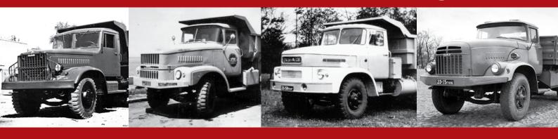
The cab is a vehicle's key attribute. The design of the very first of them derived to KrAZ truck from Yaroslavl automobile plant along with truck model was at that moment old-fashioned both in appearance and in design.
