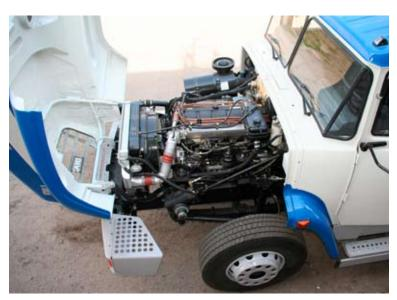
New YaMZ-6511 engine arrangement under bonnet offers easy access
