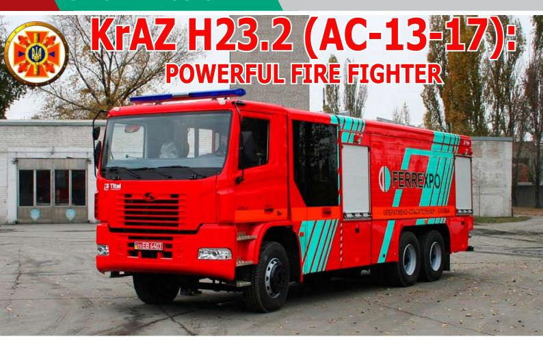
AutoKrAZ, jointly with Tital, the company specializing in production of rescue vehicles and equipment, built the new KrAZ H23.2 (AC-13-17) water tender for Eristov Mining and Concentrating Company.
