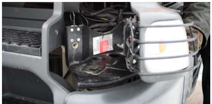
Fold-down grilled headlights simplify lamps replacement
