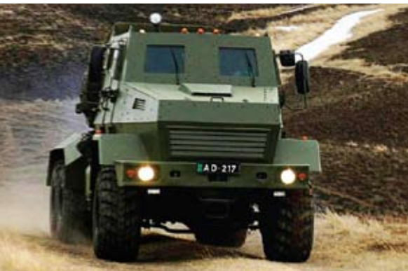
The armored RM on the KrAZ-63221 base
