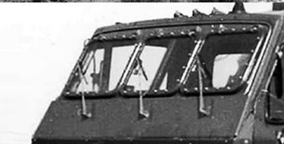
Armored cab windshield in the KrAZ-6Э6316 vehicle
