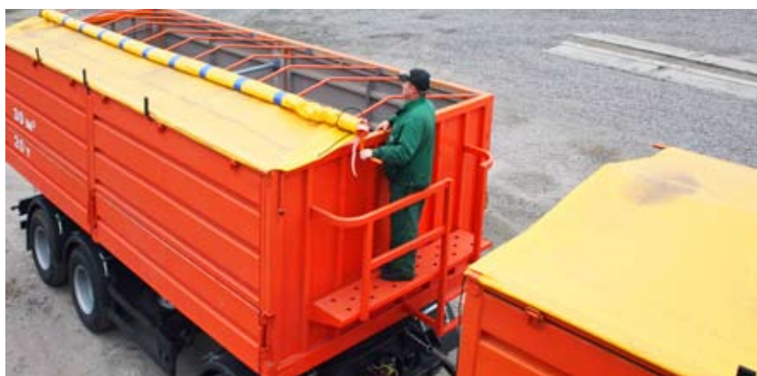
Manually moved awnings by means of special mechanisms
