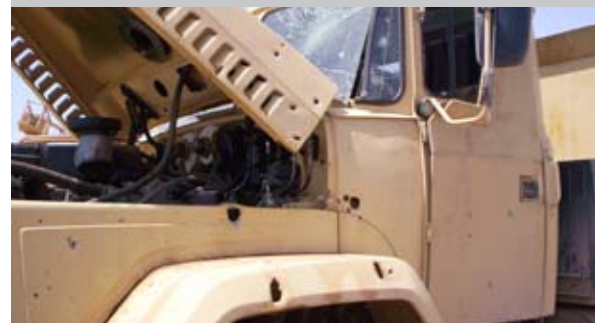
The KrAZ-6322 armored cab (local armoring with steel plates). Iraq, 2006
