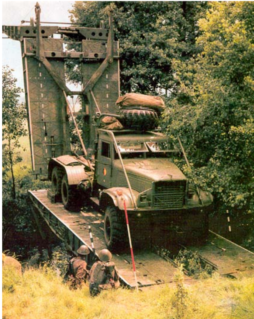
Bridge-crossing with heavy mechanized bridge on the KrAZ-255B base
