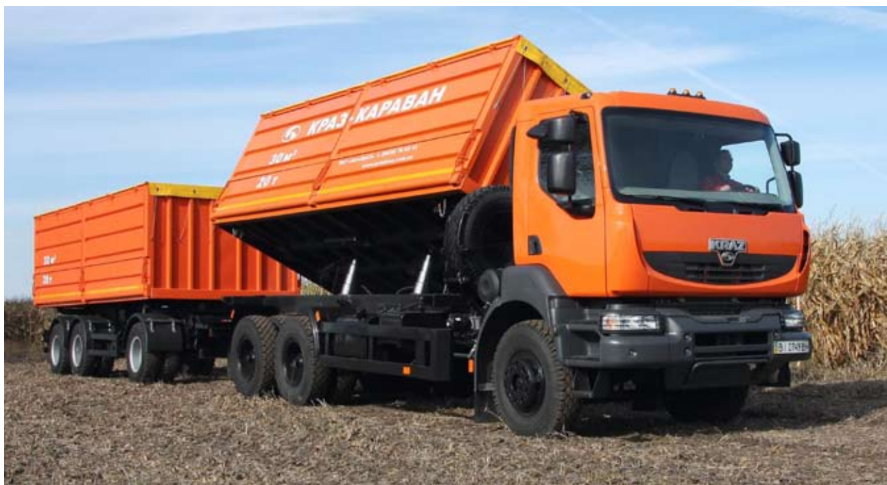
Bodies lift is carried out by the hydraulic system Penta (Italy)
