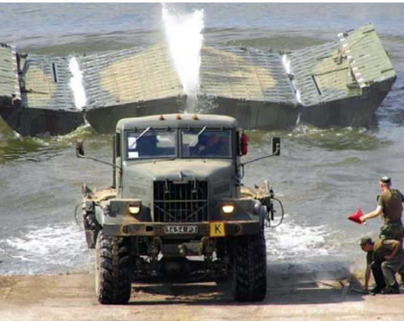
Interior bay throw off in river Float bridge set on the KrAZ-255B
