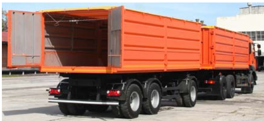
Platform tailgate with hinged doors with lateral screens and central locking
